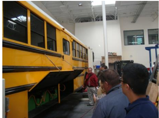
Figure 13: Battery compartment inspection.
