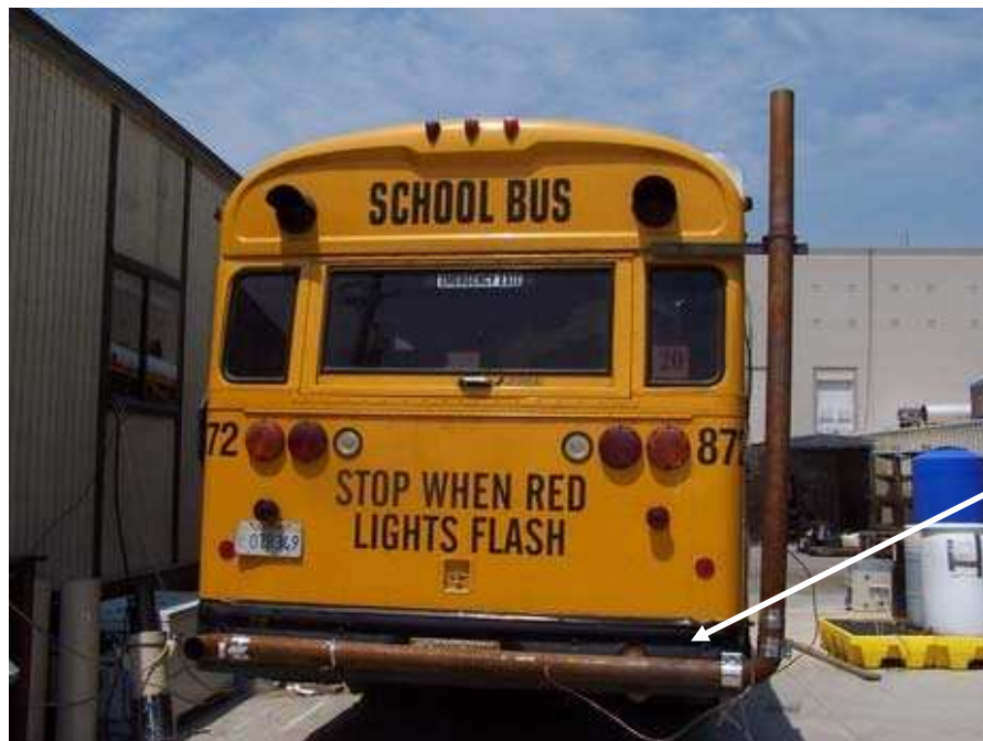
Photograph 4.2.4.3.2.1 Split exhaust configuration for self-pollution experiments. One tracer gas was released from each exhaust branch.
