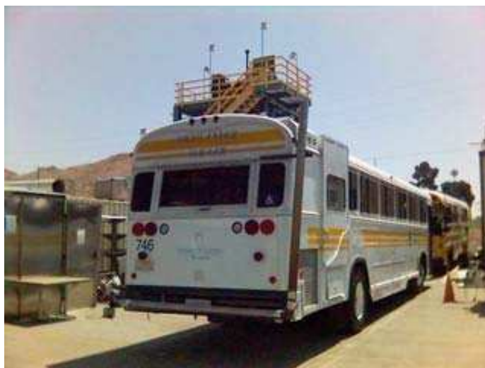
Photograph 4.2.4.4.1 Exhaust configuration for leader vehicle during leader exhaust tests to evaluate impact of following a bus with high versus low exhaust.
