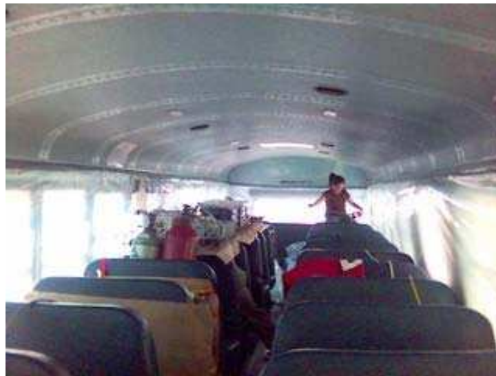
Photograph 4.2.4.2.1 Sealing passenger windows with plastic sheeting to assess contribution of window leaks to overall leaks on the bus.
